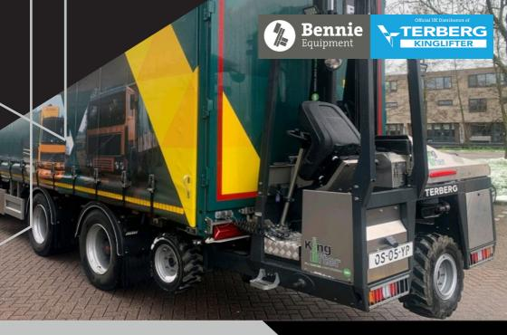
The new Lithium powered electric truck mounted forklift.
