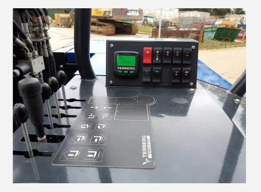
Cowl mounted levers for hydraulic functions
